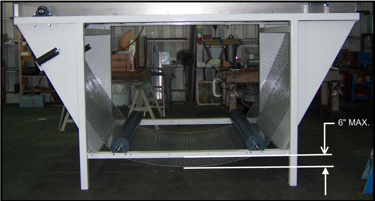
FIGURE 2.4 SIZING CHAIN SAG
