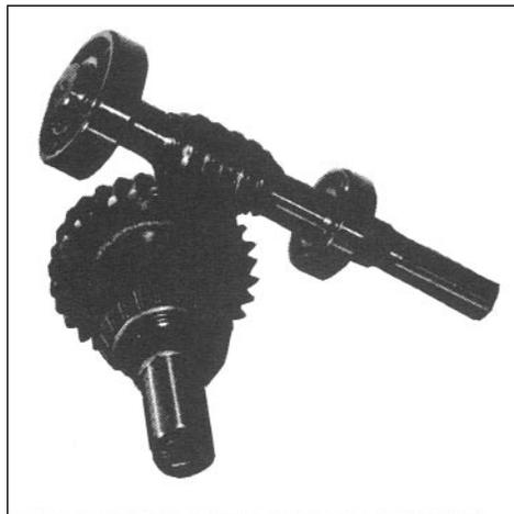
After removing worm shaft and gear shaft assemblies, clean all parts with non-flammable solvent, including tapered bearing cups pressed in bearing caps.
