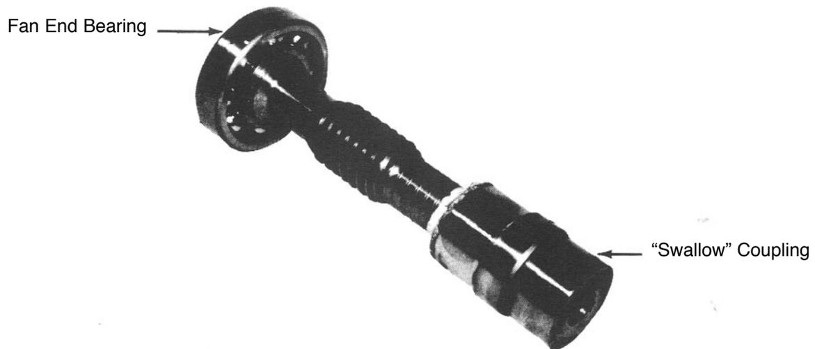
When replacing a swallow shaft worm, the worm/coupling assembly has to be ordered as a unit.
