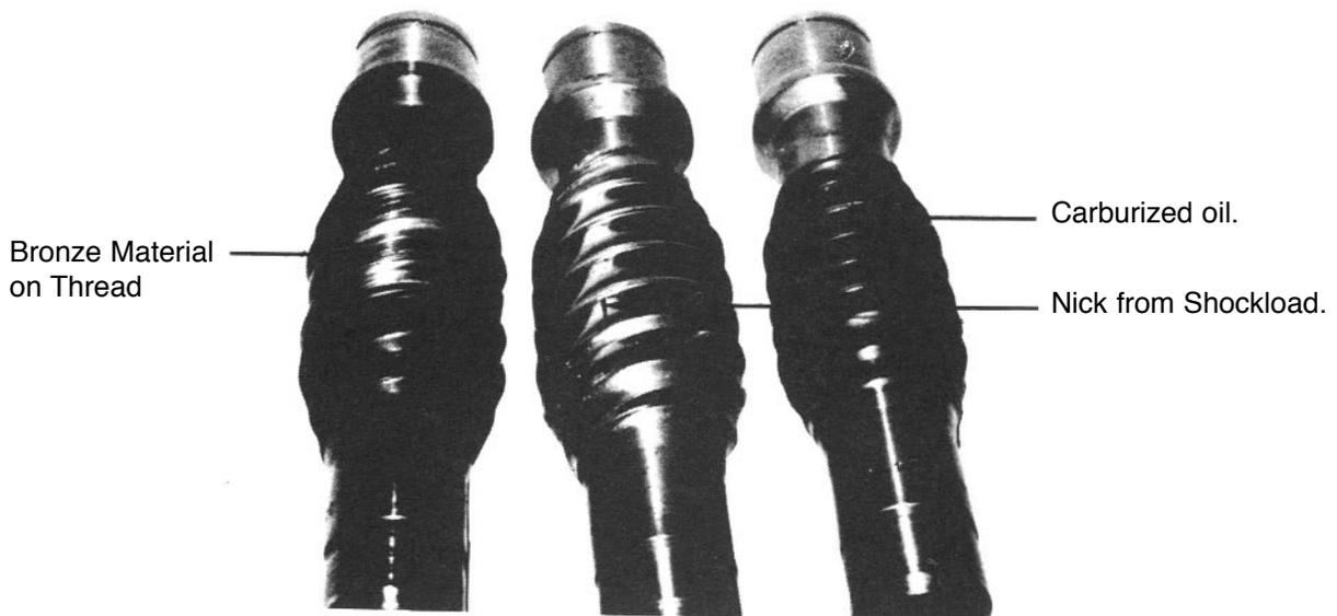
Check smoothness of worm threads. A good worm will have smooth threads. Discoloration should be noted also. Bluish tint or burnt oil indicate excessive heat, loading, incorrect lubricant, or lubrication breakdown.
